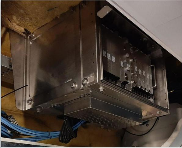
An ETCS/ATO computer (EVC) underneath the roof.
